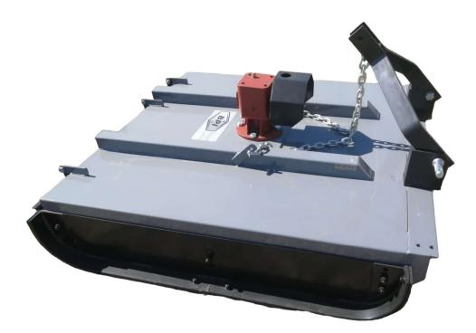
The heavy-duty slasher has been designed for all grass-cutting, bush clearing and heavy slashing operations in tough conditions, with different models having cutting widths up to 3.2m. These slashers are fitted with a heavy-duty gearbox and heavy-duty sip clutch PTO for additional machine protection. The machine works best with tractors rated from 100+kW. The blade holder system allows the blade to swing 120°.
